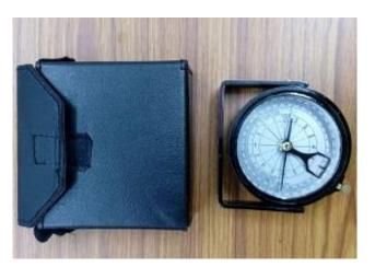
Fig. 4.1 Clinometer – Compass
